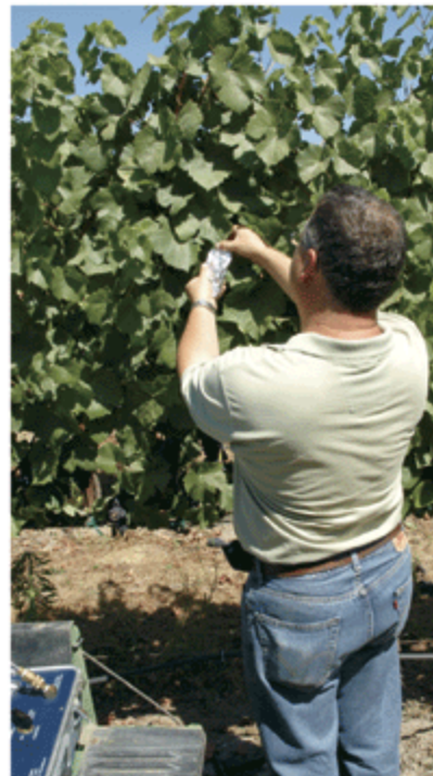
Dr. Greenspan prepares a leaf for measurement of stem water potential. A black plastic bag is wrapped tightly around the leaf, then the bag is covered with aluminum foil to avoid overheating the leaf. The bag and foil will be left on the leaf for 90 to 120 minutes.
